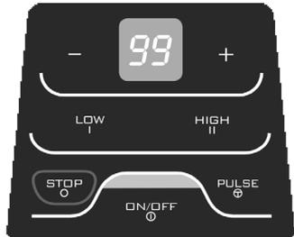
4. This blender is equipped with an electronic membrane keypad. The keypad has HIGH, LOW, STOP and PULSE buttons, as well as a 99-second countdown timer with + and – buttons. Always use HIGH speed for crushing ice. The blender can operate in two modes: timer mode and continuous mode.
