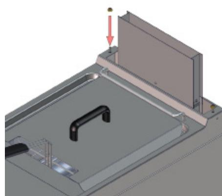
3) Mount the chimney on the prepared screws with nuts.
