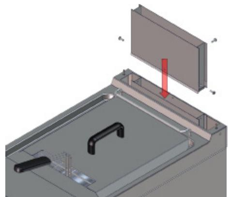
2) Place the nuts on the prepared screws, but do not tighten them.
