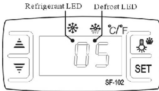
1. Adjust the temperature: Press the button **SET**, the set temperature is displayed. Push the button **▲** Or **▼** to modify and store the displayed value. Push the button **SET** to exit the setting and display the cold room temperature.
