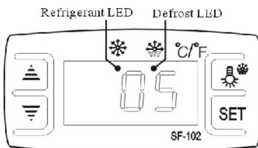
2. Adjust the temperature: Press the button **SET**, the set temperature is displayed. Push the button **▲** Or **▼** to modify and store the displayed value. Push the button **SET** to exit the setting and display the cold room temperature.
